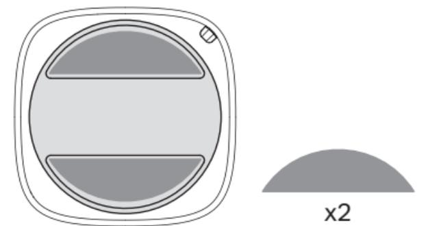
b. Magnetically attach the sensor to metallic surfaces.
